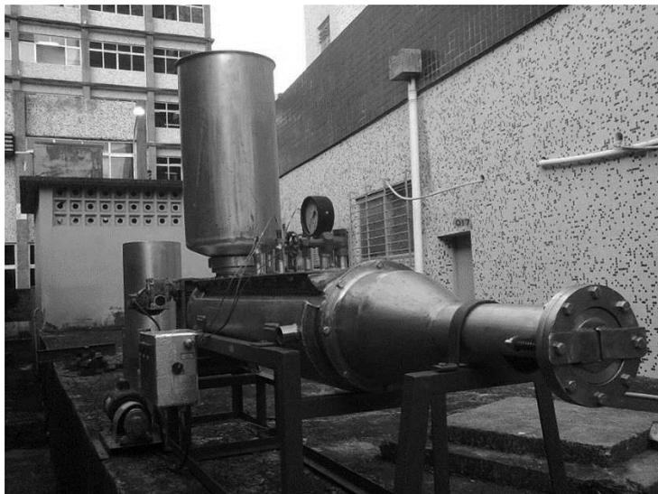
Figure 2. Photograph of continuous reactor with mobile helical element on bench scale
