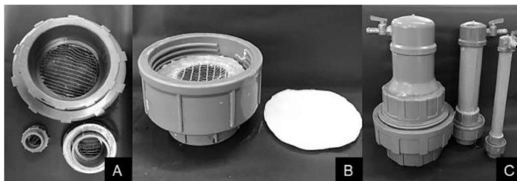
Fig. 1. Inner diameters (25, 50 and 100 mm) of PVC filters (A); BC membrane previously prepared with same diameter as filter coupled to filtration system (B) and filtration systems in PVC (C).
