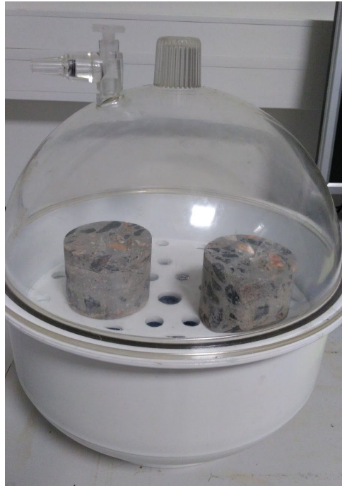
Figure 83. Desiccator where the sample was placed when it was removed from the greenhouse.
