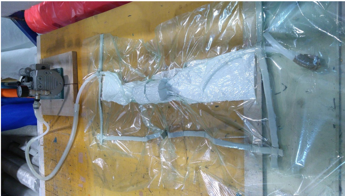
Figure 84. Vacuum pump on removal of all air from the system for apparent porosity test.
