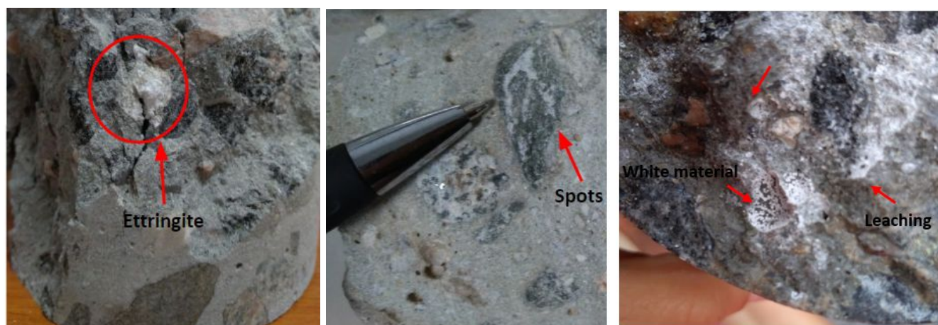
Figure 51. Symptoms of the expansion mechanisms found: a) Pores fullled with ettringite; b) Spots in the aggregate; c) White material in the pores and Leaching.
