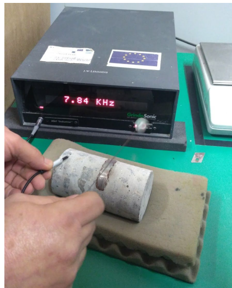
Figure 54. Part of a steel bar in the concrete specimen (AM-1B) during the dynamic modulus test.
