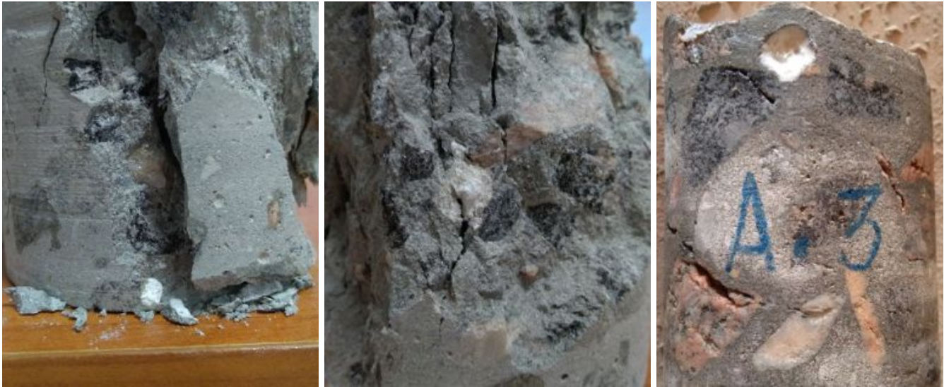
Figure 70. Pores completely filled with ettringite crystals: a) and b) Concrete sample after compressive rupture; c) Concrete sample after extraction.
