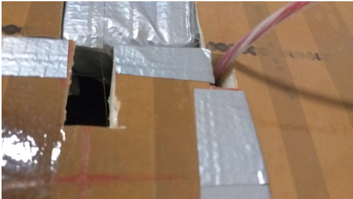
Figure 55: Openings to Allow the Passage of the Sensors (Author, 2020)
