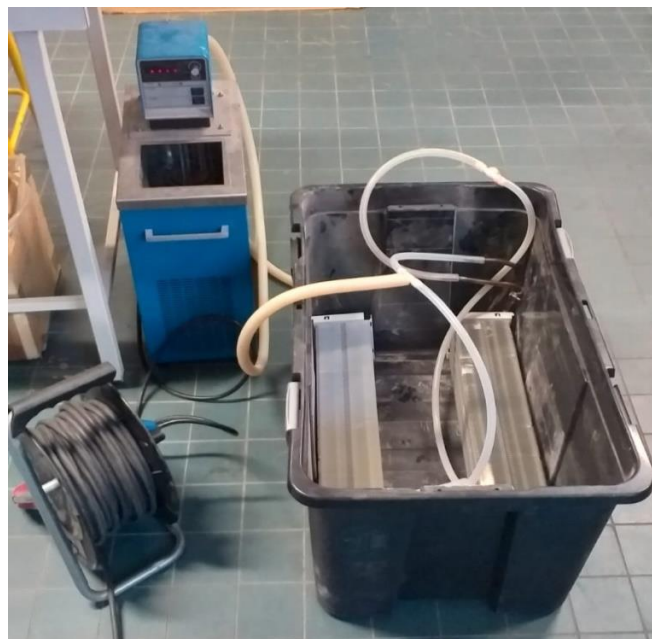
Figure 42: Tank with the heating system (Author, 2020)
