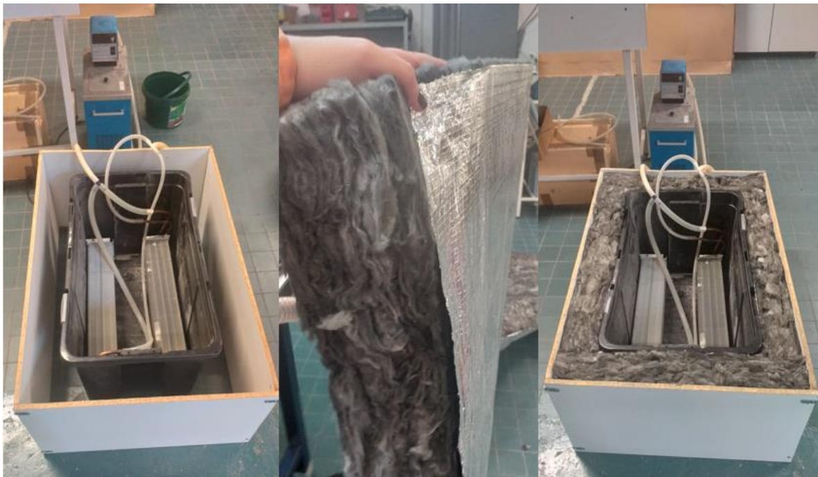
Figure 44: Thermal insulation of the tank (Author, 2020)
