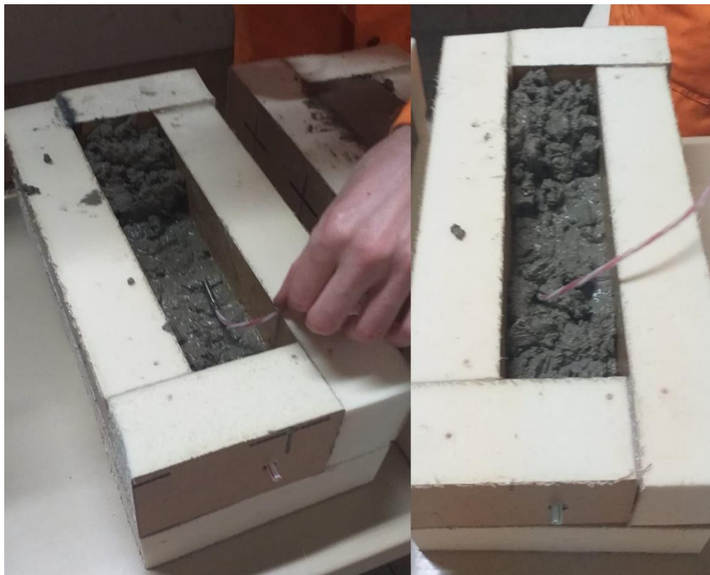
Figure 51: Temperature sensor insertion (Author, 2020)
