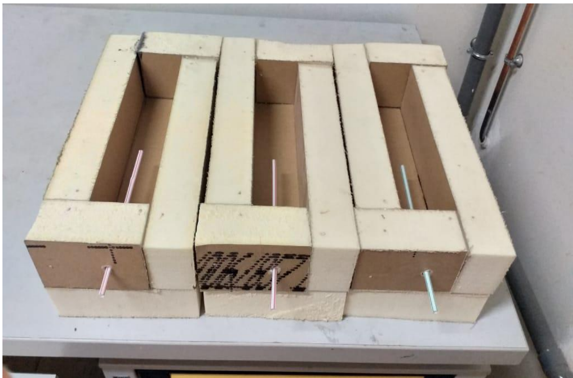
Figure 49: Molds with hole for sensor insertion (Author, 2020)
