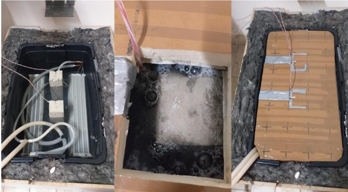
Figure 54: Concrete prisms inside the tank (Author, 2020)
