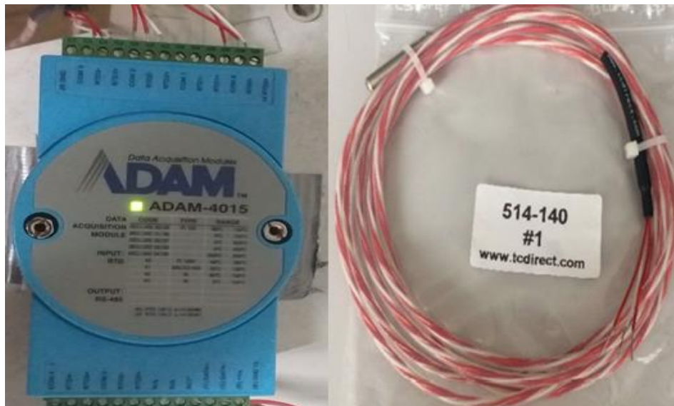
Figure 47: Temperature measurement system and temperature sensor (Author, 2020)
