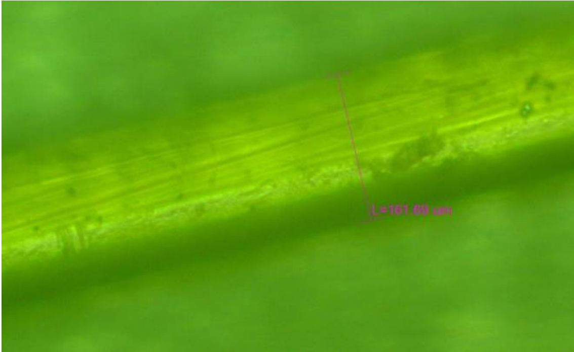
Figure 68: Optical fiber without contact with the NaOH solution (Author, 2020)
