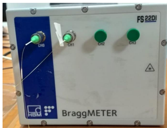
Figure 46: HBM FS22 DI Industrial BraggMETER optical interrogator (Author, 2020)
