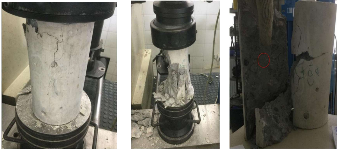
Figure 20 – Typical failure mode of compression test specimens.
