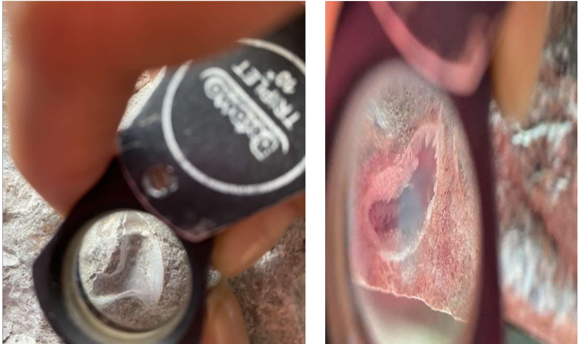
Figure 18 – Crystals of the expansive gel can be seen through a magnifying glass.
