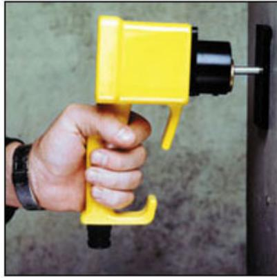
**Figura 1 - Windsor Probe Test System**
