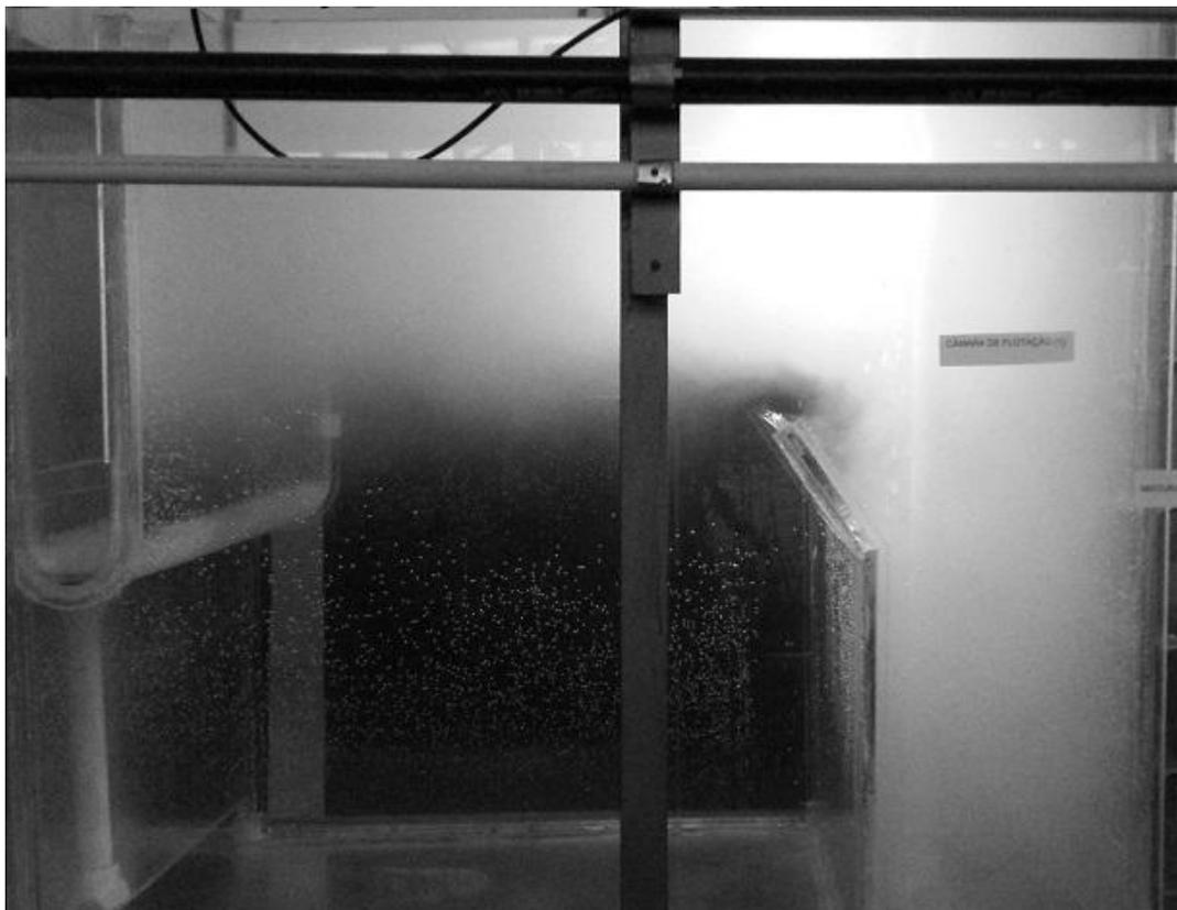
Figure 6: External view of microbubbles distribution in prototype flotation chamber
