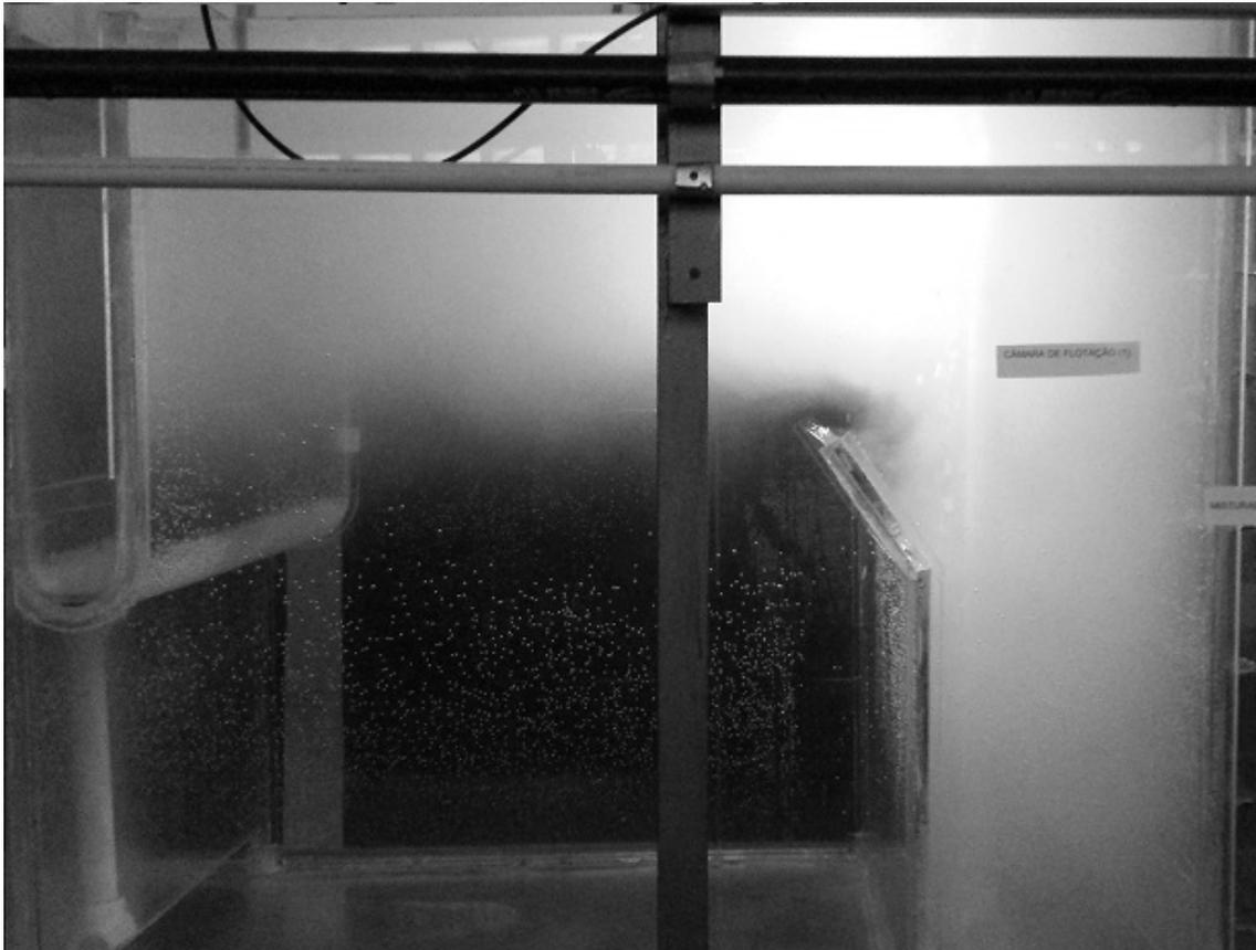
Figure 5: Photograph showing distribution of microbubbles in flotation chamber of DAF prototype
