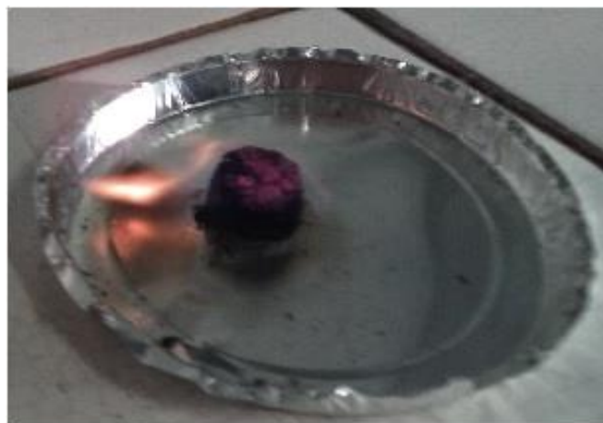
Figure 3: Experiments of briquettes burning with the aid of a blowtorch for visual identification of fouling levels as a function of the content of gypsum waste
