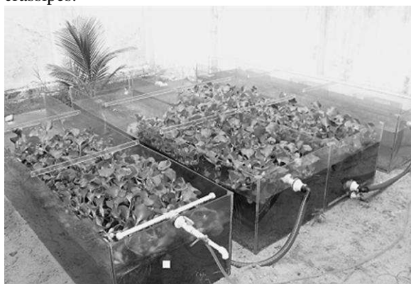
Fig 2. Wetlands constructed in transparent polycarbonate with floating macrophytes
