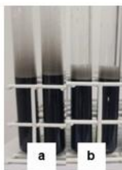
Figure 5. Dispersion of India ink by foam of sodium cocoyl isethionate (a) and foam of biosurfactant produced by Starmarella bombicola ATCC 22214 (b).
